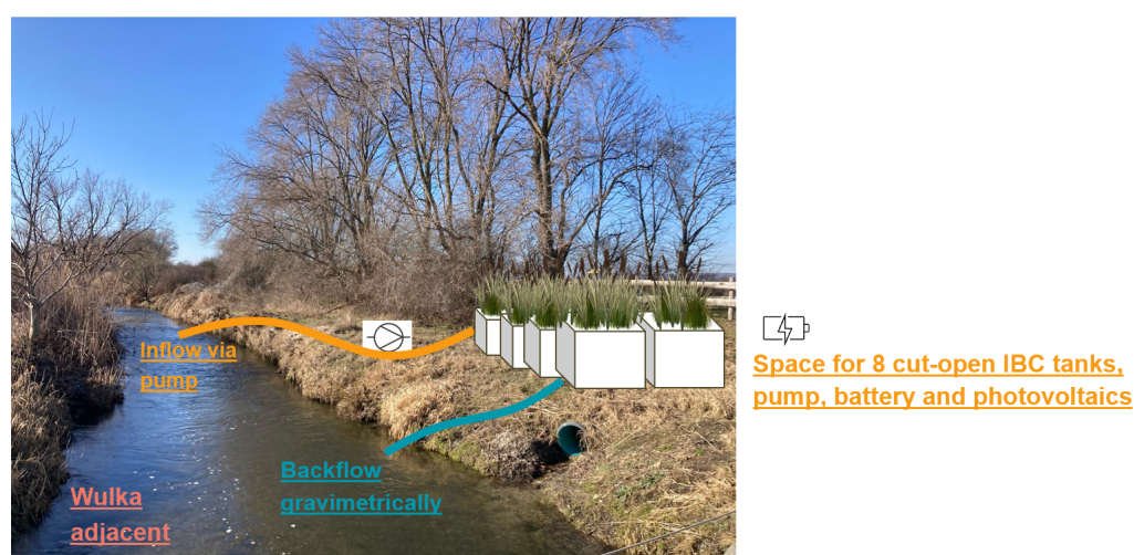
Figure 4 Sketch of the setup adjacent to the Wulka with 8 IBC tanks, water intake and backflow.
